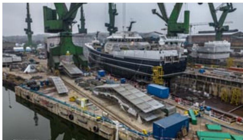
The steel-hulled Høgaberg has three continuous decks with a long forecastle and boat decks
